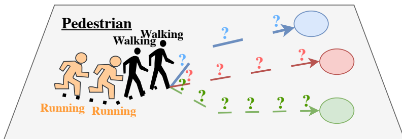
Figure 1.5: Joint Trajectory and Action Prediction (TAP) task: given the observed trajectory, observable class, and fine-grained actions augmenting the observed trajectory, the task involves simultaneously predicting the future trajectory and the corresponding sequence of fine-grained actions.
