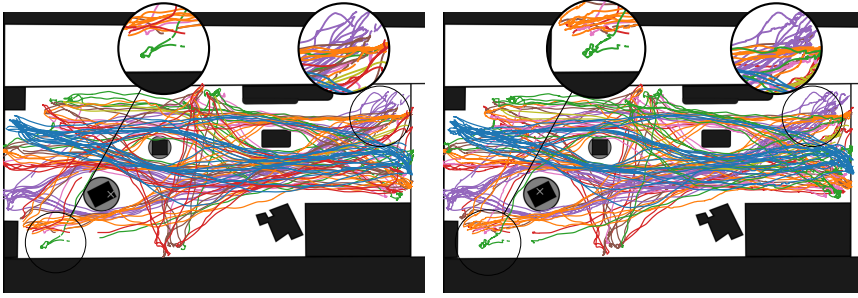
Figure 3.8: Filtering methods in a 4-minute recording from Scenario 1. Left: trajectories filtered using the most reliable marker. Right: trajectories filtered using the average of the tracking locations of each marker. Although the average tracking markers method provides longer tracks, it induces jerkier trajectories, especially near the boundaries of the motion capture volume (e.g., bottom left and top right).
